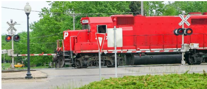
In a railroad quiet zone, safety controls are upgraded in exchange for less horn use.
