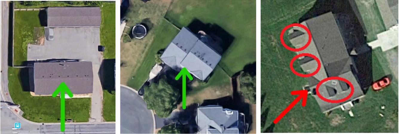
**Building Orientation:** Buildings should be oriented to maximize a south facing roof, or flat roof sections with quality south light access. Building orientation and configuration should maximize future solar panel access to sunlight. Buildings should be oriented with their long axis East and West, making the longest face of the building the South facing plane
