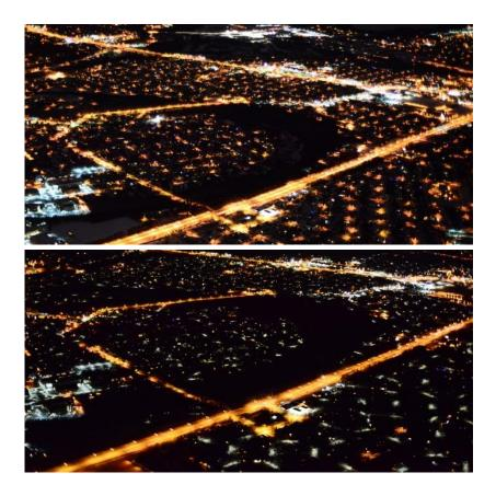
Images courtesy of Xcel Energy. Before and after photos of a high pressure sodium street light retrofit to LEDs. The utility's city-wide conversion saved the City about \$40,000, 900,000 kWhs, 1 million lbs. of CO<sub>2</sub>, and reduced light pollution.
