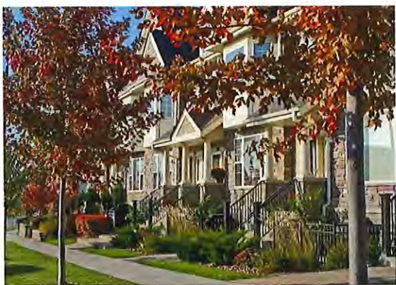
The porches, stairs and landscaped setbacks of these townhouses demarcate private, semi-private and public spaces while providing an attractive environment for walking and “defensible space.”
